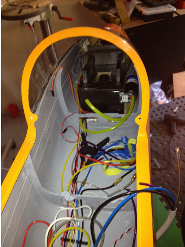
Photo 4 – air lines colour coded and run to the centre area of the component boards. The Speed brake air lines have been run to this spot too.
