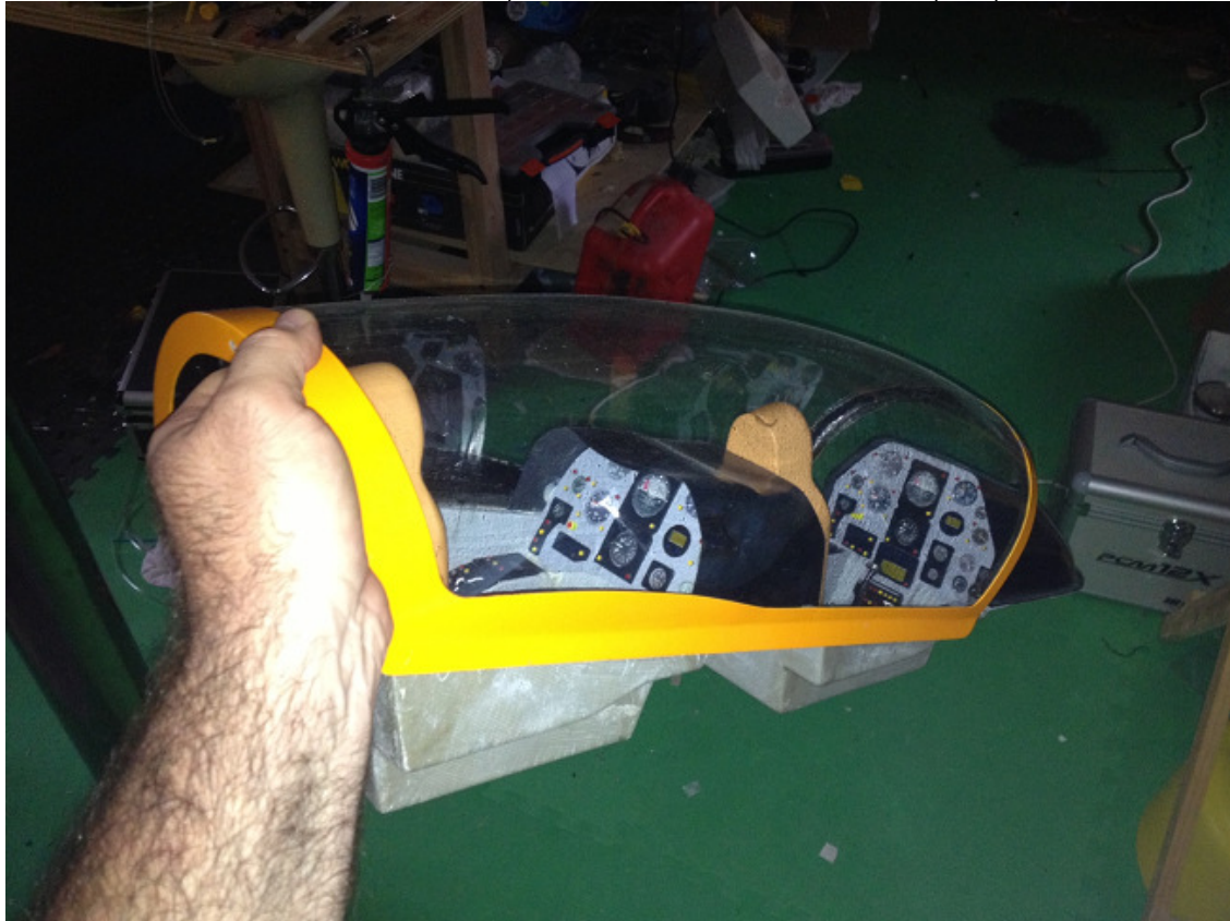
Photo 11 – trim the sides of the cockpit area such that the tubs drop in place
