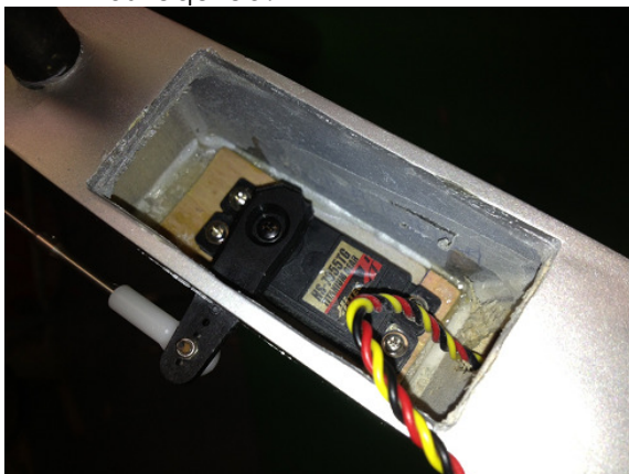
Photo 5&6 – Rudder Servo and push rod.
