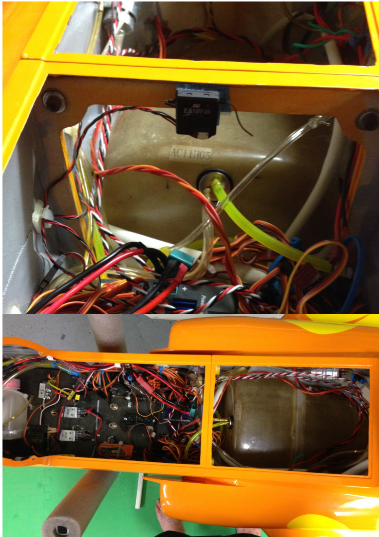
Photo 2 – Smoke Tank Layout added for Deisel. Used some saddle tanks around ducting.
