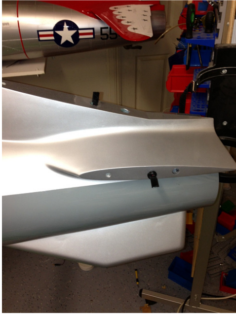
Photo 7 – Rear section with the tailplane and vertical stab removed.
