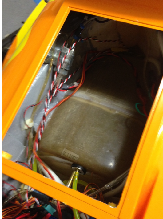
Photo 3 – air tanks tucked into the leading edges of the fuse section.
